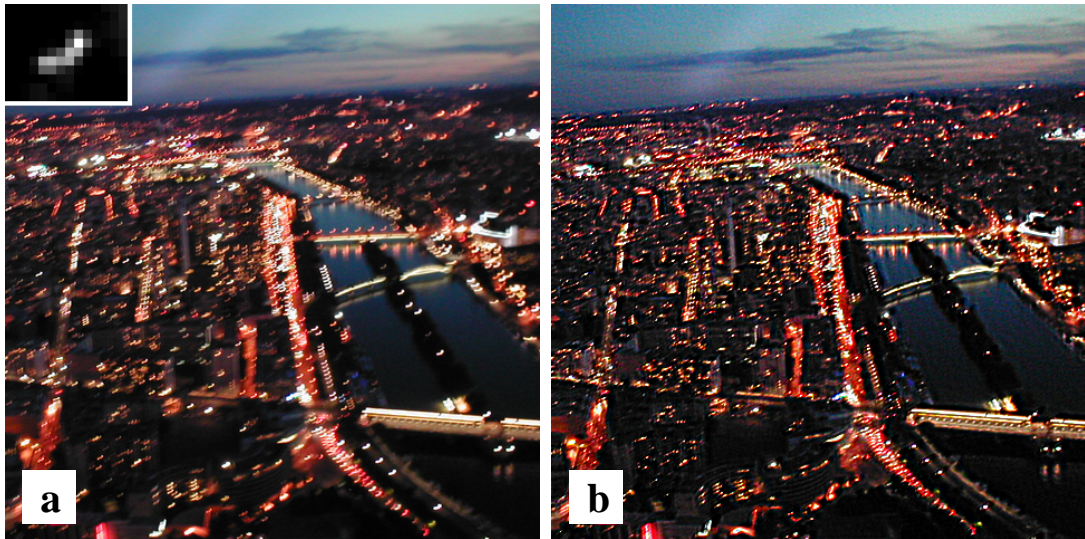
Figure 7: (a) Colour photograph (Paris from Eiffel Tower) blurred during acquisition, 480 \times 480 pixels. Insert shows approximate point-spread function used for deconvolution (same as in Figure 1, eight times enlarged). (b) Richardson-Lucy deconvolution, 20 iterations.
