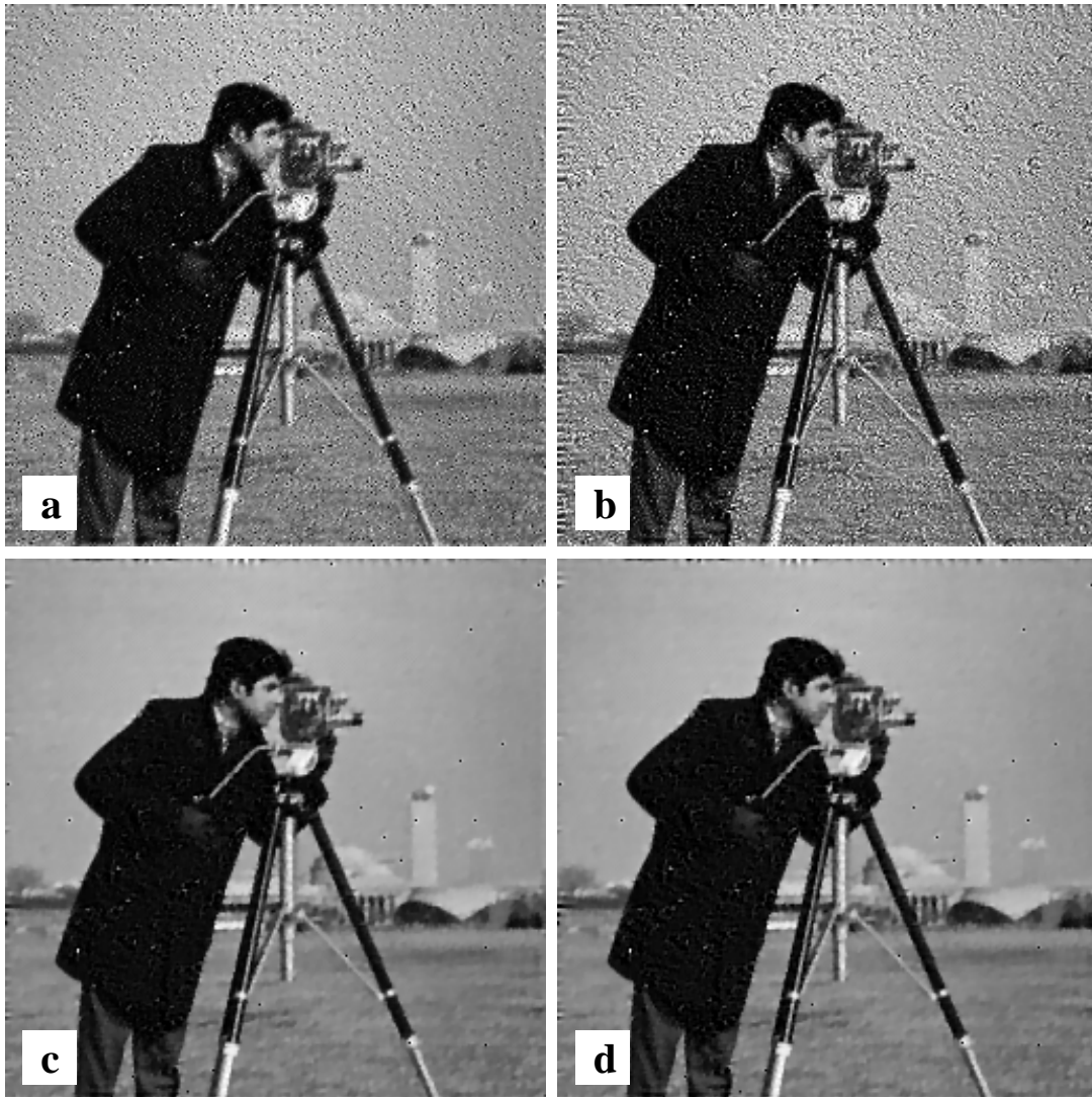
Figure 4: (a) Image from Figure 1(b) deblurred by 50 iterations of robust RL, SNR: 6.42 dB. (b) 200 iterations of robust RL, SNR: 4.00 dB. (c) 200 iterations of robust and regularised RL (19) with regularisation weight \alpha = 0.005 ; SNR: 14.41 dB. (d) Same but 2000 iterations; SNR: 14.21 dB.
