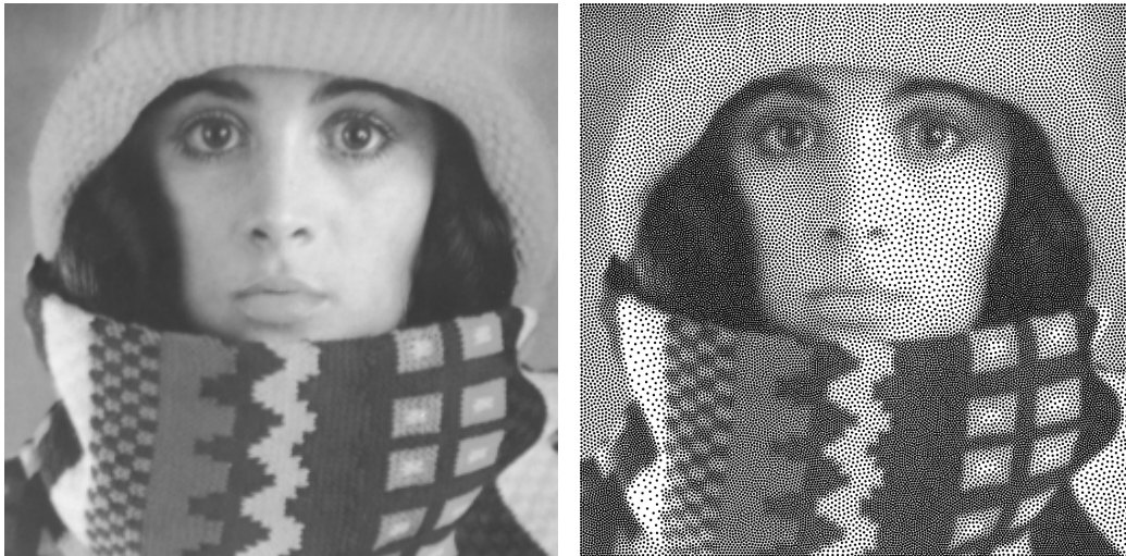
Figure 2: Test image Trui , 256 \times 256 pixels. Left: Original. Right: Stippling with 30150 dots. This image serves as a basis for our quantitative evaluation. Runtime on GeForce GTX 480: 33.6 ms per iteration, or 6.72 s for 200 iterations.
