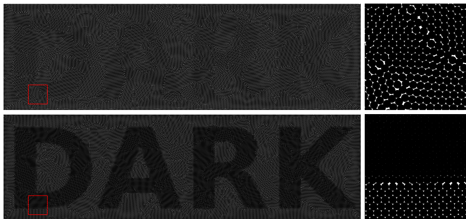
Figure 10: Illustration of grey-value correction in dark image areas. Shown are halftoning results of an image containing the word “DARK” with grey value 0 on a background with grey value 10 ( 320 \times 95 ). Top: Standard halftoning. Bottom: With proposed grey-value correction. Note that the difference between both images might be indistinguishable on some output devices, e.g. due to ink bleeding.
