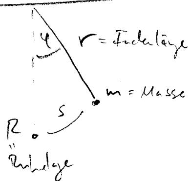
$$s(t) = r \varphi(t) \text{ Auslenkung,} \\ \Rightarrow s''(t) = r \varphi''(t)$$
