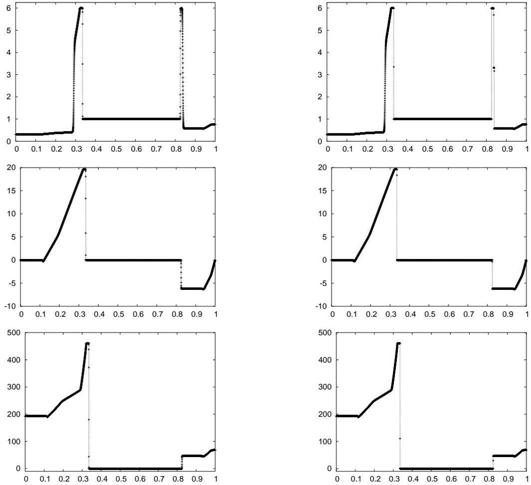
Figure 7: Approximation of the Woodward-Colella blast wave test case by the NT scheme. Comparison of states (left column) before and (right column) after filtering. **Top row:** density. **Middle row:** velocity. **Bottom row:** pressure.
