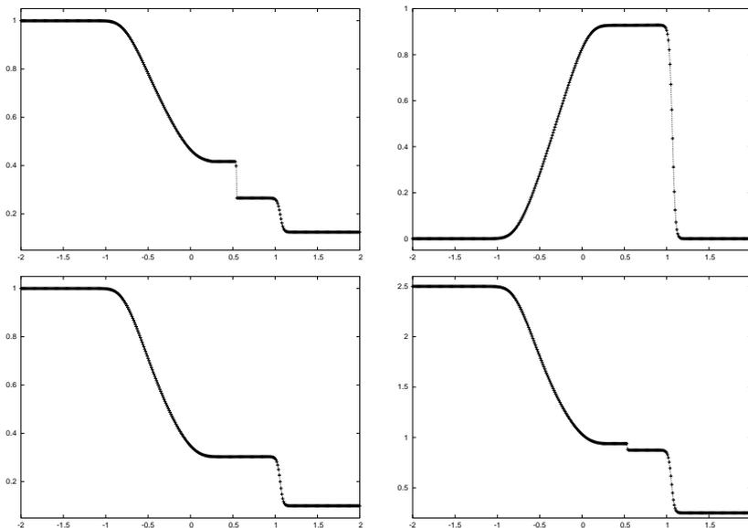
Figure 4: Selective filtering of the contact discontinuity. **Left column:** density (top) and pressure (bottom). **Right column:** velocity (top) and total energy (bottom).
