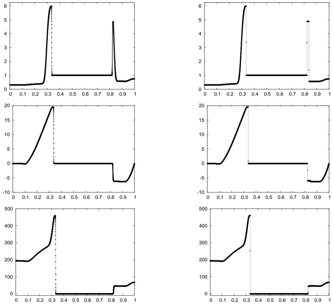
Figure 6: Approximation of the Woodward-Colella blast wave test case by the mLF scheme. Comparison of states (left column) before and (right column) after filtering. **Top row:** density. **Middle row:** velocity. **Bottom row:** pressure.
