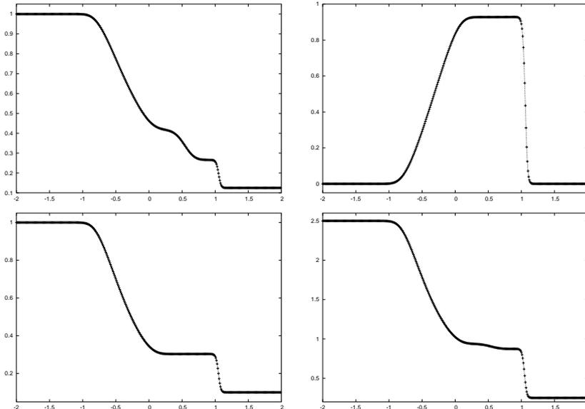
Figure 2: Diffusive artefacts within a first-order numerical approximation of the shock tube problem. **Left column:** density (top) and pressure (bottom). **Right column:** velocity (top) and total energy (bottom).
