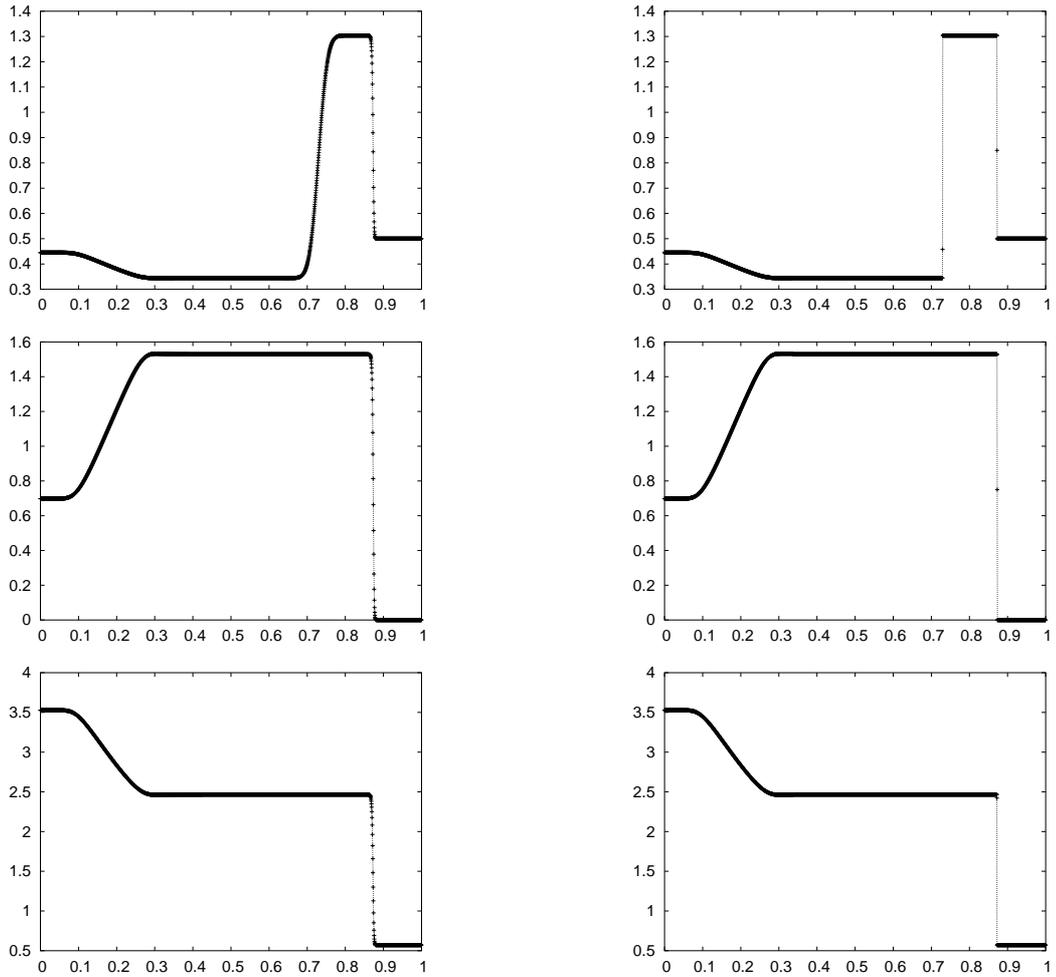
Figure 8: Approximation of the Lax test case by the mLF scheme. Comparison of states (left column) before and (right column) after filtering. **Top row:** density. **Middle row:** velocity. **Bottom row:** pressure.
