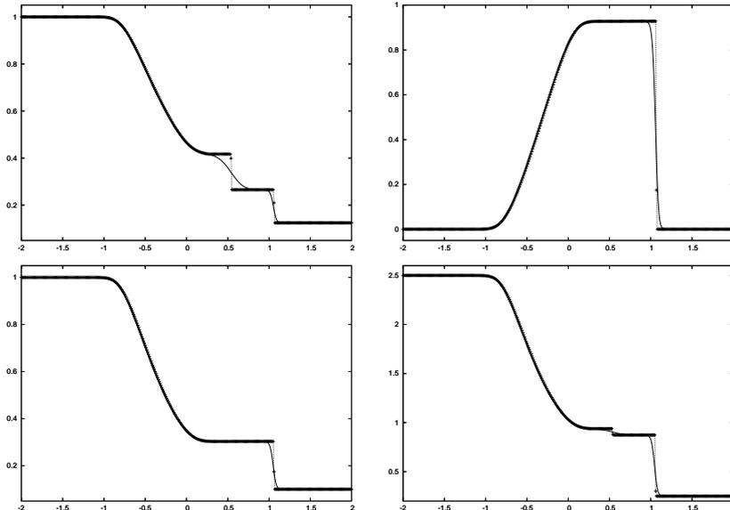
Figure 5: Filtering of all discontinuities. **Left column:** density (top) and pressure (bottom). **Right column:** velocity (top) and total energy (bottom).
