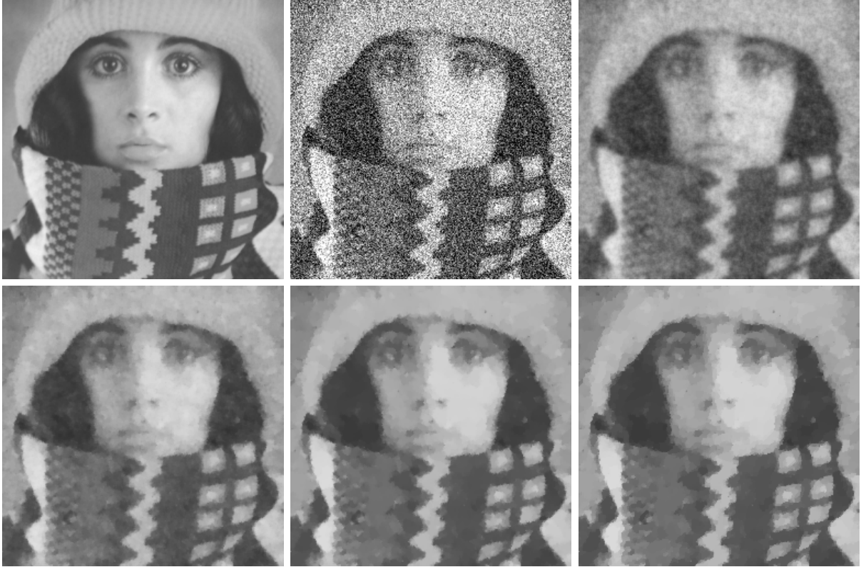
Figure 1: Denoising experiment. (a) Top left: Test image, 256 \times 256 pixel, range [0, 255] . (b) Top middle: Degraded by additive Gaussian noise with zero mean and standard deviation \sigma = 49.49 . (c) Top right: Whittaker-Tikhonov regularization ( \mu = 0 ) of the noisy image (b) with regularization parameter \alpha = 5.8 , yielding an MSE of 155.82. (d) Bottom left: Result for \mu = 1.5 and \alpha = 54 . MSE = 122.96. (e) Bottom middle: Result for \mu = 20 and \alpha = 1410 . MSE = 114.70. (f) Bottom right: Result for TV-regularization with \alpha = 86 . MSE = 124.48.
